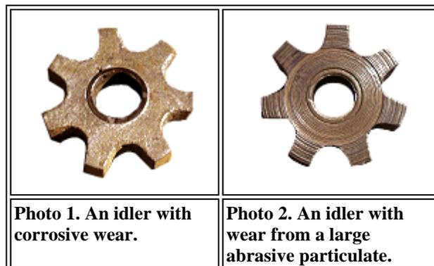
Typical corrosive applications can be found in almost every industry, but they are particularly common in the chemical and paper industries. Typical abrasive applications are found in the paint and coatings industry, the printing industry, magnetic oxide tape coating, and a variety of other processes.
