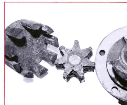
FIGURE 1. Parts from a Viking Internal Gear Pump deliberately run at excessive speeds on an accelerated water test. The appearance is typical of that caused by severe cavitation.
